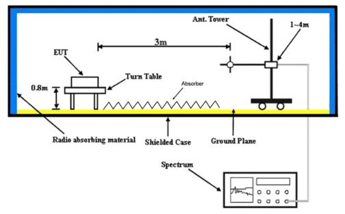
Note: According to EN 55032 standard, cables on the RGP must be insulated.
