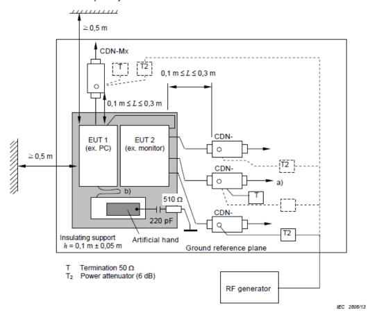
a) Only one of the CDNs not used for injection shall be terminated with 50 Ω, providing only one return path. All other CDNs shall be configured as decoupling networks.
